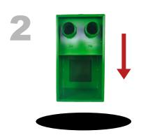
Lower unit body vertically into manhole.
