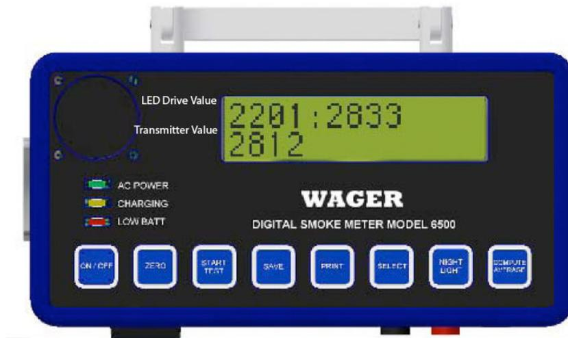
The goal of the optic alignment is to have the TX and RC values to be equal and around 2800.
